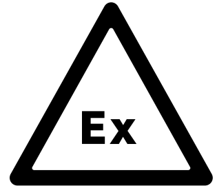
Fig. 0B - Warning sign for areas subject to the risk of explosion - Directive 99/92/EC
